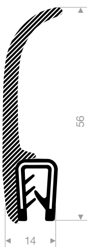
VR24500876 pvc + sponge rubber clamping range 1-3 mm roll length 25 meter
