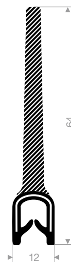
VR24500865 pvc + sponge rubber clamping range 1-2,5 mm roll length 50 meter
